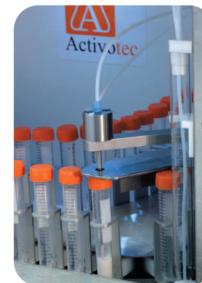
Fresh amino acids and pre-activation vessel
