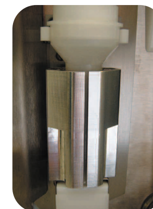
Heated reactor • Ambient to +70 °C • Cooling • Increased coupling efficiency
